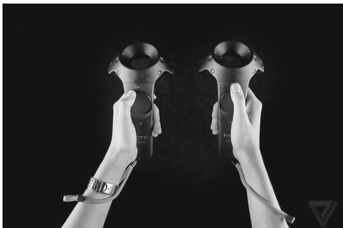
**Fig. 2.** HTC Vive controllers with haptic feedback
