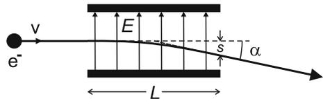
which is independent of the mass  $m$  but depends on the energy  $W$ . Noting that the tangent to the parabola at the exit point intersects the undeflected orbit at  $x = L/2$ , the deflection angle becomes  $\alpha = \arctan(2s/L)$ . This independence of mass is the reason why a transverse electric field can be used as an *energy filter* to sort out particles of same energy independent of their mass.
