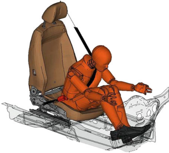
Fig. 12 Car seat crash simulation [18]. Published with kind permission of ©Fraunhofer SCAI 2016. All Rights Reserved
