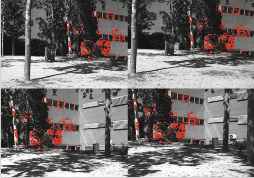
Fig. 2.4 Some of the SIFT correspondences in two consecutive stereo image pairs and their covariance. The ellipses represent iso-uncertainty curves plotted at a scale of 3 standard deviations
