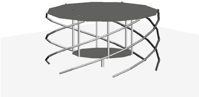
**Fig. 1.** Disk-loaded monopole with a 6-wires helical cage
