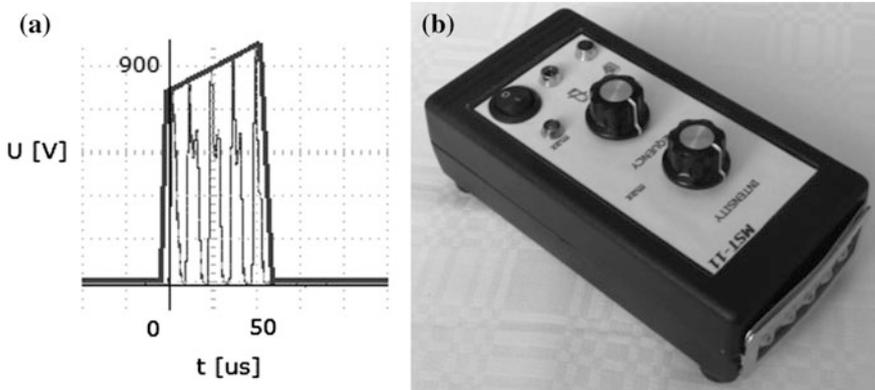
**Fig. 3** The Microstimulator (b) and the shape of pulses on Microstimulator's output (a) [23]. The recording was made during the real measurement using oscilloscope. The therapeutic pulse is marked clearly as an envelope of the burst
