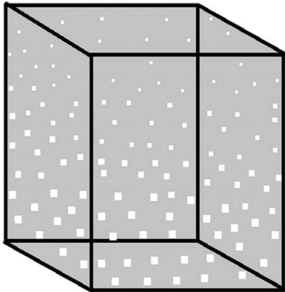
gradient of the FGM, on the other hand, is produced by varying the pore sizes or the pore shape, or both.
