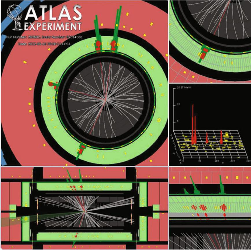
**Fig. 1.3** The decay of a Higgs boson to four electrons as detected by the ATLAS experiment. The electrons are visible as *straight* lines in the inner tracking system and large *energy deposits* in the electromagnetic calorimeter. Reprinted with permission from [4]
