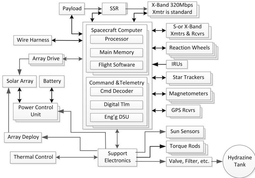
**Fig. 4** Integrated electronic system of WorldView satellites
