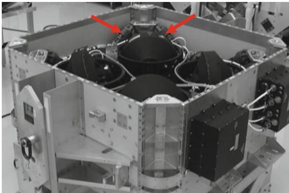
**Fig. 6** Chandra X-ray vibration isolator
