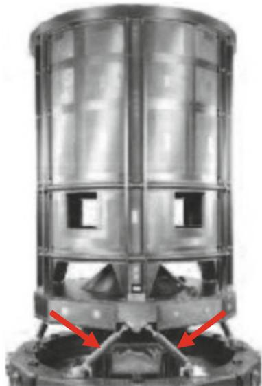
flexible appendages. As shown in Fig. 9, a damper was used on the root of the solar array of the Hubble telescope, which effectively reduces the amplitude of sloshing and improve the attitude stability [10].
