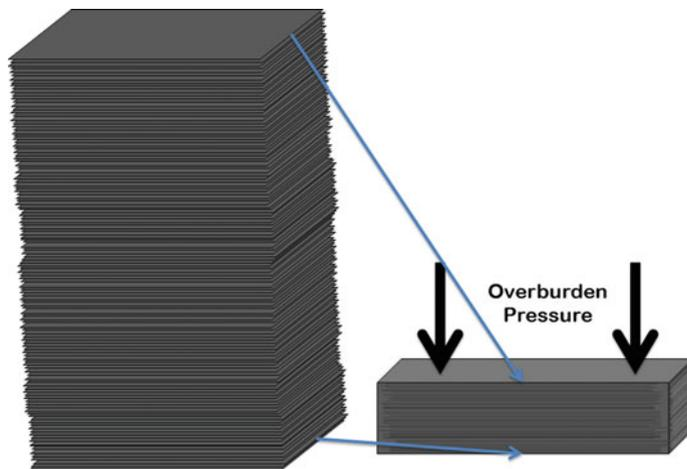
**Fig. 2.7** Schematic of the nature of the SNFN in shale outcrops and its potential shape when subjected to overburden pressure
