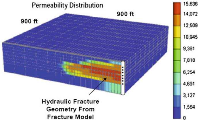
Fig. 2.8 Example of explicit hydraulic fracture (EHF) modeling [28]
