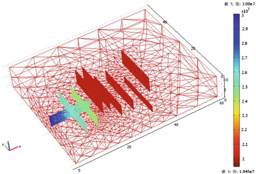
**Fig. 2.4** Hydraulic Fracture propagation distribution at time-step 20 [11]
