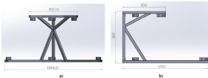
**Fig. 3** A 3D model of the proposed mechanical structure with main sizes in mm: **a** front view; **b** side view
