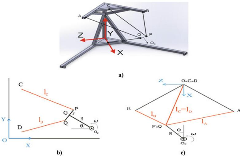
**Fig. 4** Kinematic schemes: **a** a 3D view with reference frame and location of cable attachments; **b** X-Y (flexion-extension) plane; **c** X-Z (adduction-abduction) plane
