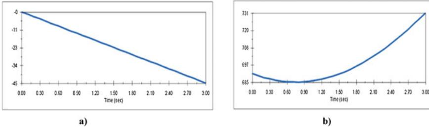
**Fig. 6** Plot outputs from the simulation in Fig. 5: **a** angular displacement ( $^{\circ}$ ) of the forearm over time (s); **b** distance (mm) of point  $O_C$  (attachment of the wrist) relative to point P (attachment of the first two cables) over time (s)
