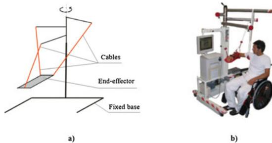
**Fig. 10** MariBot rehabilitation robot: **a** Structural diagram; **b** design of the prototype
