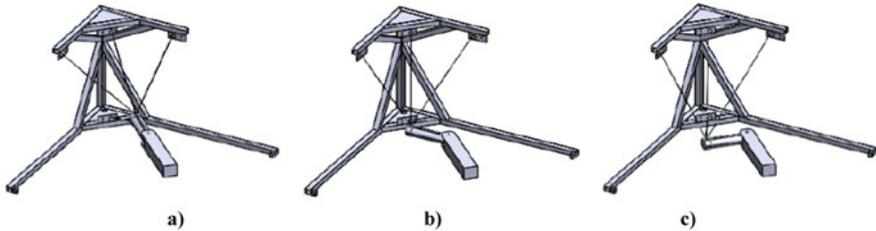
**Fig. 5** Snapshots taken from a Solidworks Motion simulation of the adduction training movement: **a** forearm at 0°; **b** forearm at 45°; **c** forearm at 90°
