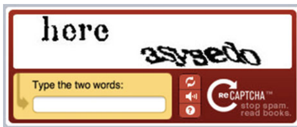
Fig. 1 Re-CAPTCHA: the computer not only tests whether its interlocutor is human or not (by asking him to decipher the twisted text on the right) but also asks him what is the word on the left (that it could not recognize via Optical Character Recognition because it was badly printed)
