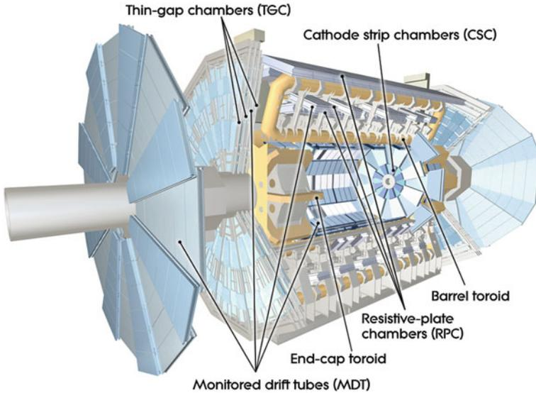
Fig. 2.5 Layout of the ATLAS muon system. From [7]
