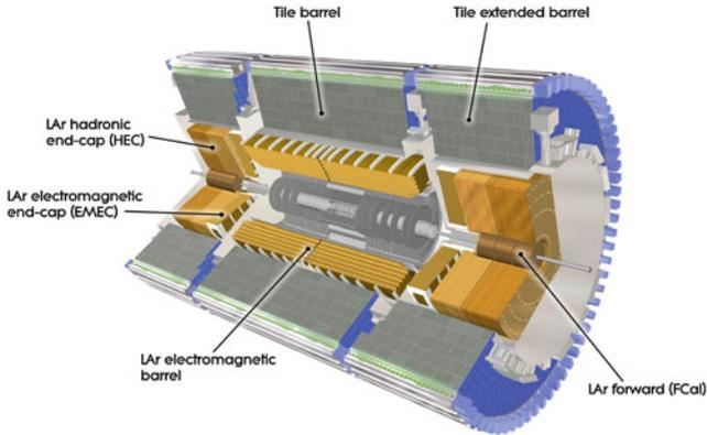
**Fig. 2.4** Layout of the ATLAS calorimeter system. From [7]
