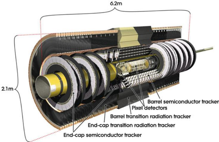
**Fig. 2.3** Layout and sub-components of the ATLAS Inner Detector. From [7]
