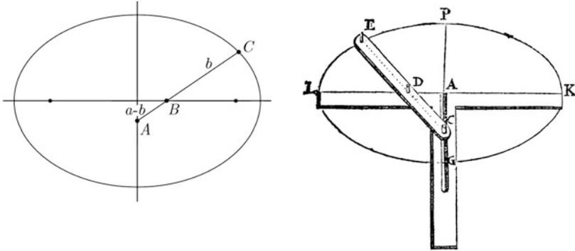
■ **Fig. 2.13** Archimedes' trammel (right: van Schooten (1659), KBR VH 8.040 A)
