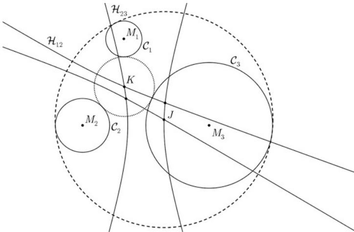
■ **Fig. 2.8** Three circles, in solid lines, are given. The hyperbolae which are the loci of the centre of circles tangent to  $C_1$  and  $C_2$  on the one hand and  $C_2$  and  $C_3$  on the other are drawn. The intersection point  $A$  is the centre of a circle externally tangent to the three circles (dotted line). The intersection point  $B$  is the centre of a circle for which the given circles are internally tangent (dashed line)
