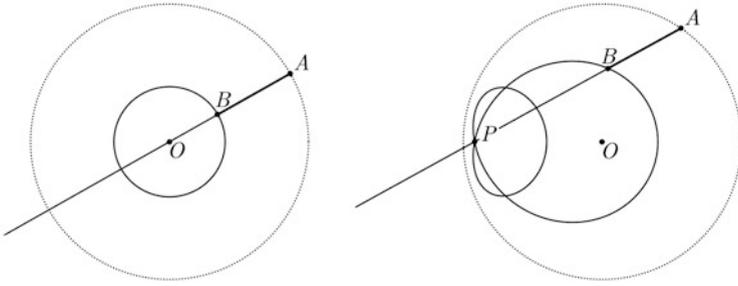
**Fig. 2.22** The locus of  $B$  with  $A$  generated by a neusis in which the directrix is a circle. *Left* if the pole coincides with the centre of the circle, *right* if the pole and the centre do not coincide
