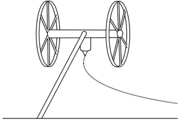
Point  $D$  is attached to  $KL$  and can move along this slat. Put  $\|DE\| = b$ . As  $D$  is moved along  $KL$   $E$  traces out an ellipse.
