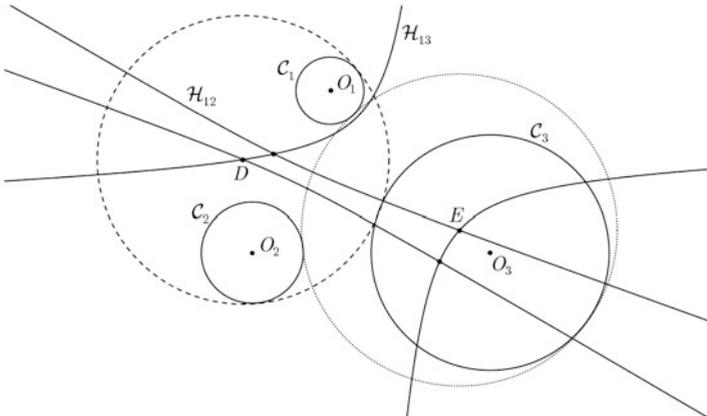
**Fig. 2.10** Another solution to Apollonius' problem. The hyperbolae which are the loci of the centres of circles tangent to  $C_1$  and  $C_2$  on the one hand, and  $C_1$  and  $C_3$  on the other, are drawn. The intersection point  $D$  is the centre of a circle externally tangent to one circle and internally tangent to two (*dashed line*). The intersection point  $E$  is the centre of a circle externally tangent to two circles and internally tangent to one (*dotted line*)
