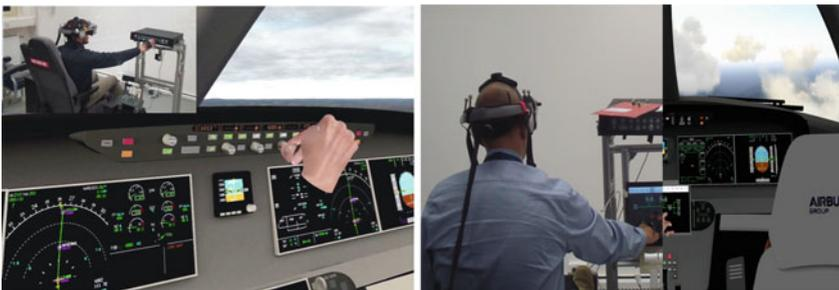
Fig. 3 Interaction with hardware components in the VRFS
