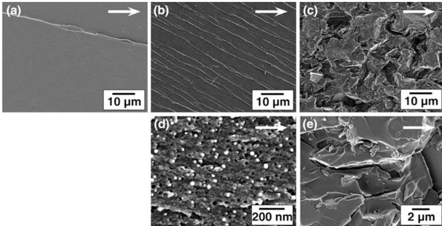
**Fig. 2.3** Fracture surfaces (SEM) of the different nanocomposites in the region of stable crack growth, **a** neat epoxy, **b** and **d** nano-SiO<sub>2</sub> nanocomposites, **c** and **e** O/K-hect nanocomposites. The direction of crack propagation is indicated by the *white arrows*
