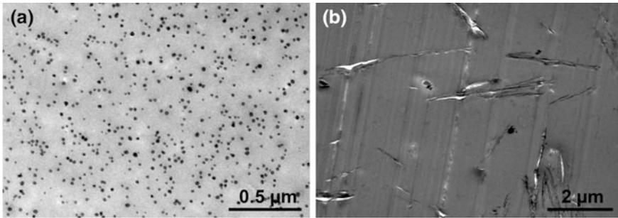
**Fig. 2.1** TEM micrographs of the nanocomposites filled with **a** 2.7 vol% SiO<sub>2</sub>, and **b** 2.2 vol% O/K-hect
