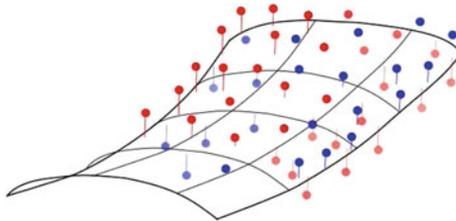
**Fig. 4** Before boresight calibration, soundings from two overlapping swaths may not fit on a quadratic surface. In this example, the two point clouds do not match with any quadratic surface. In our approach, the quadratic surface and the boresight angles are adjusted in order to fit the overlapping point clouds
