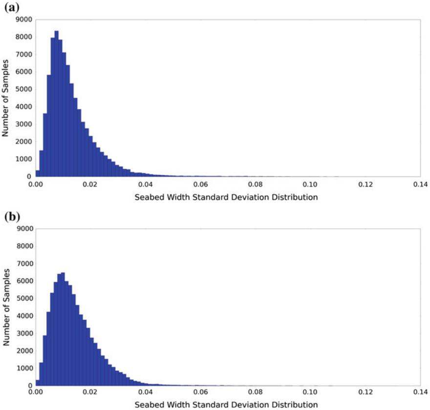
**Fig. 5** From the two histograms, one can see that the automatic boresight method (a) provides a better global fit of overlapping data. Indeed the plot shows number or samples versus the adjustment error. **a** seabed width standard deviation histogram with estimated boresight angles correction. **b** seabed width standard deviation histogram with Patch-test boresight angles correction
