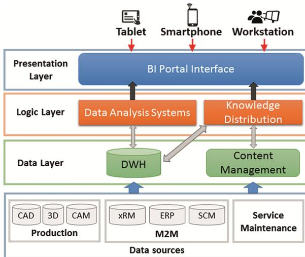
Fig. 1. Generalised BI-enabled Industry 4.0 System (non-cloud-based)
