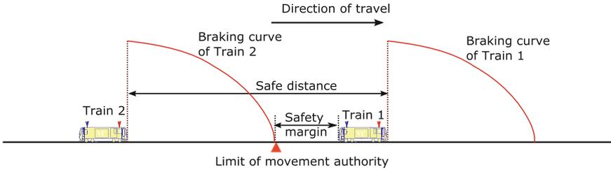
**Fig. 2.4** The principle of a pure MBS system
