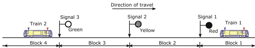
**Fig. 2.3** Three aspect fixed block signaling system
