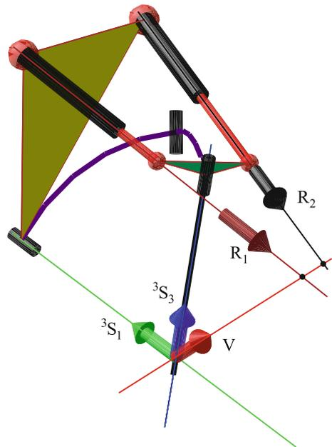
**Fig. 4** A singular configuration of the robot and the plane defined by two joint axes  ${}^3S_1$  and  ${}^3S_3$
