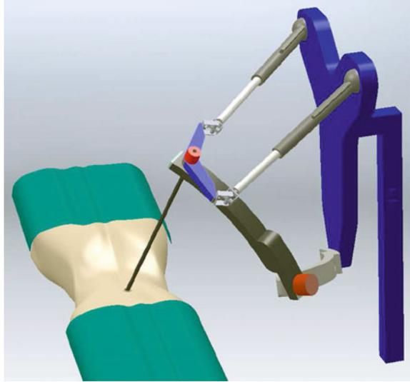
has three limbs (legs) and 2SPU1RRR structure. A CAD model of the considered hybrid robot is shown in Fig. 1.
