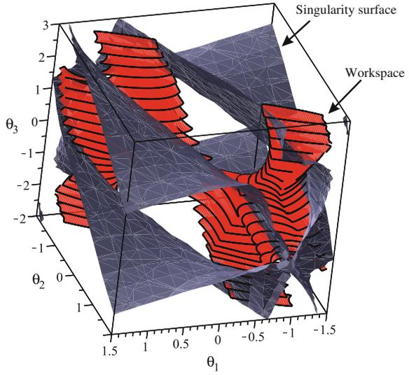
**Fig. 6** The singularity curve and workspace boundary of the robot for  $\theta_3 = 0$
