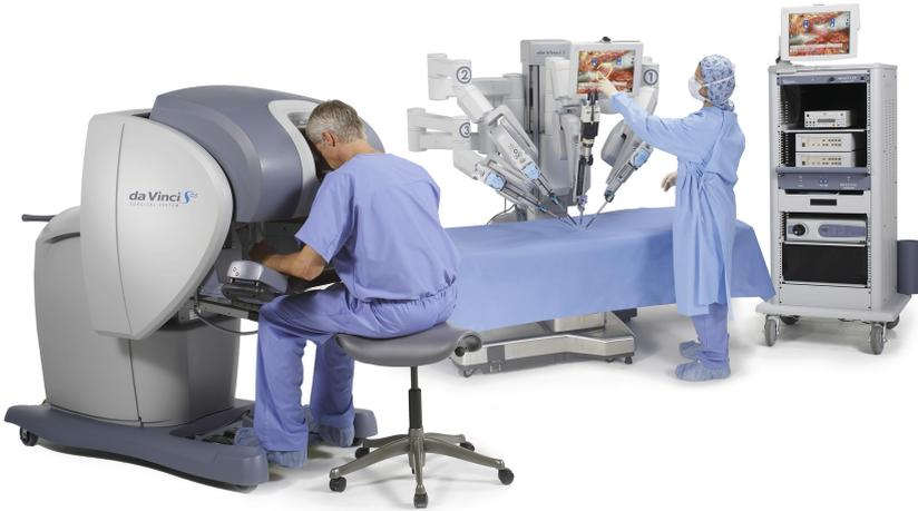
**Fig. 1.** Setup of a da Vinci S HD Surgical System. Left: surgeon (in our case the trainee) operating the console. Center: patient cart and assistant (in our case the instructor) using the telestration feature of a touch screen. Right: vision cart. Copyright 2015 Intuitive Surgical, Inc.
