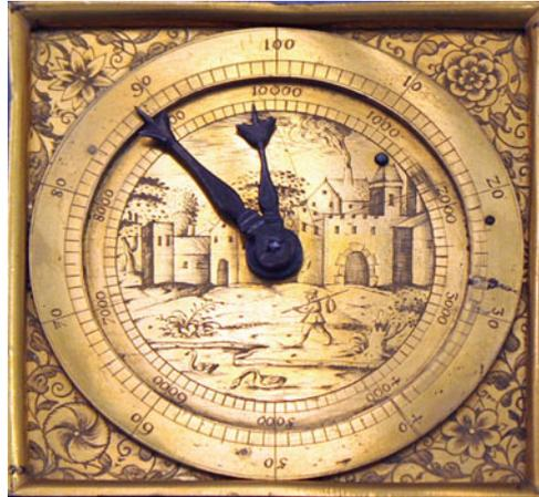
**Fig. 2.12** Han Kemper evaluated the traditional type of pedometer, based on a pocket watch mechanism. He found that sometimes it counted two steps rather than one during jogging, and that it failed to record at all during slow walking
