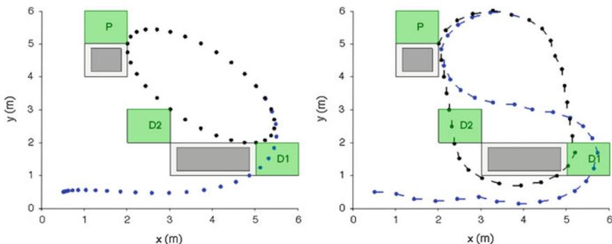
**Fig. 1** Illustration of a problem instance. The task is to repeatedly visit regions  $P$ ,  $D1$ , and  $D2$ , where *dark* regions are obstacles that must be avoided. Representative trajectories for a quadrotor (*left*) and nonlinear car (*right*) are shown with the prefix (*blue*) and suffix (*black*)
