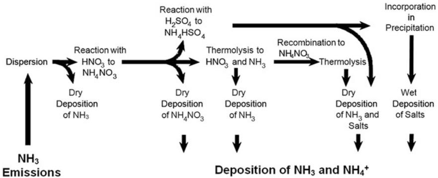
Fig. 2.9 Emission, dispersion, vertical and horizontal transport, chemical reactions, and deposition of ammonia and ammonium (Amended, translated and adopted from Dämmgen and Erisman 2002), where NH<sub>3</sub> is ammonia; HNO<sub>3</sub> is nitric acid; NH<sub>4</sub>NO<sub>3</sub> is ammonium nitrate; NH<sub>4</sub>HSO<sub>4</sub> is ammonium hydrogen sulfate; and H<sub>2</sub>SO<sub>4</sub> is sulfuric acid
