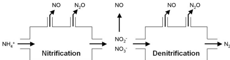
**Fig. 2.5** Formation and release of N<sub>2</sub>O and NO by nitrification and denitrification (Amended by Reinhardt-Hanisch 2008 adopted from Colbeck and Mackenzie 1994)
