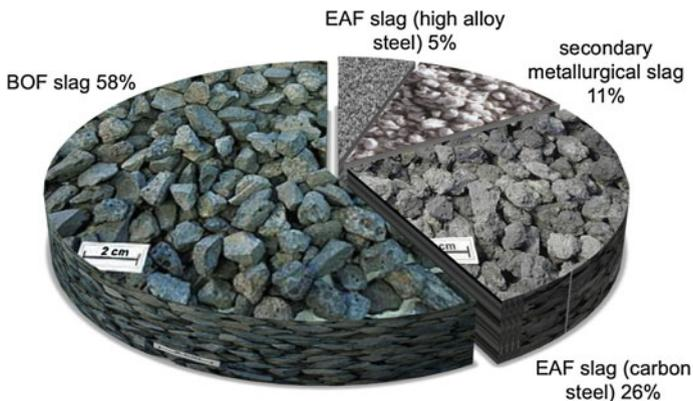
Fig. 2.3 Steel slag production in Europe [72]
