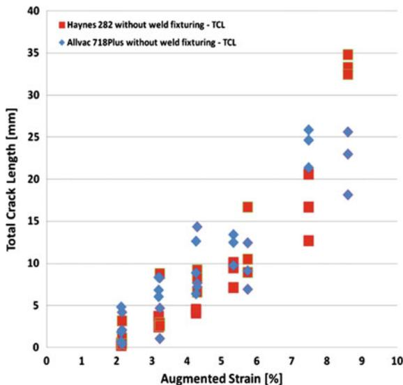
Fig. 10 Comparison in cracking response between Haynes<sup>®</sup> 282<sup>®</sup> and ATI 718Plus<sup>®</sup> in varestreint testing using both test configurations
