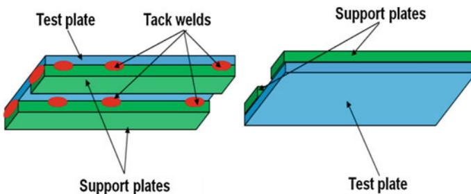
**Fig. 4** Varestraint testing configurations in the present study
