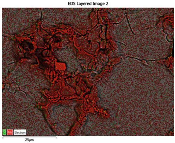
Fig. 12 SEM-EDS elemental map of ATI 718Plus<sup>®</sup> revealing enrichment of Nb and C
