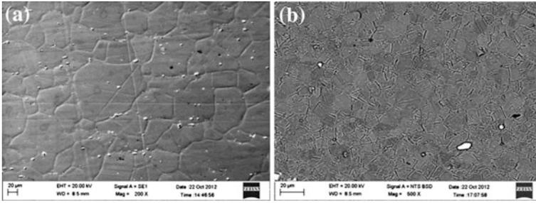
**Fig. 5** The microstructure of as-received material: **a** Haynes® 282® (GS 65 µm, HV 215) and **b** ATI 718Plus® (GS 10 µm, HV 330)
