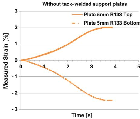
**Fig. 6** Example of strain measurement in pure bending with a target strain of  $\sim 2\%$  using a test plate thickness of 5 mm and radius of 133 mm (R133) with support plates lying free on top of the test plate. The *solid line* reveals measurements from the *top side* of the test plate, whereas the *dotted line* represents measurements from the *bottom side* of the same test plate
