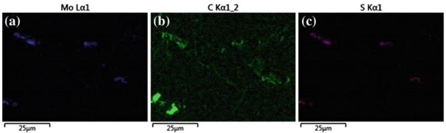
Fig. 14 SEM-EDS elemental maps of a liquated grain boundary in Haynes<sup>®</sup> 282<sup>®</sup> revealing enrichment of a Mo, b C and c S
