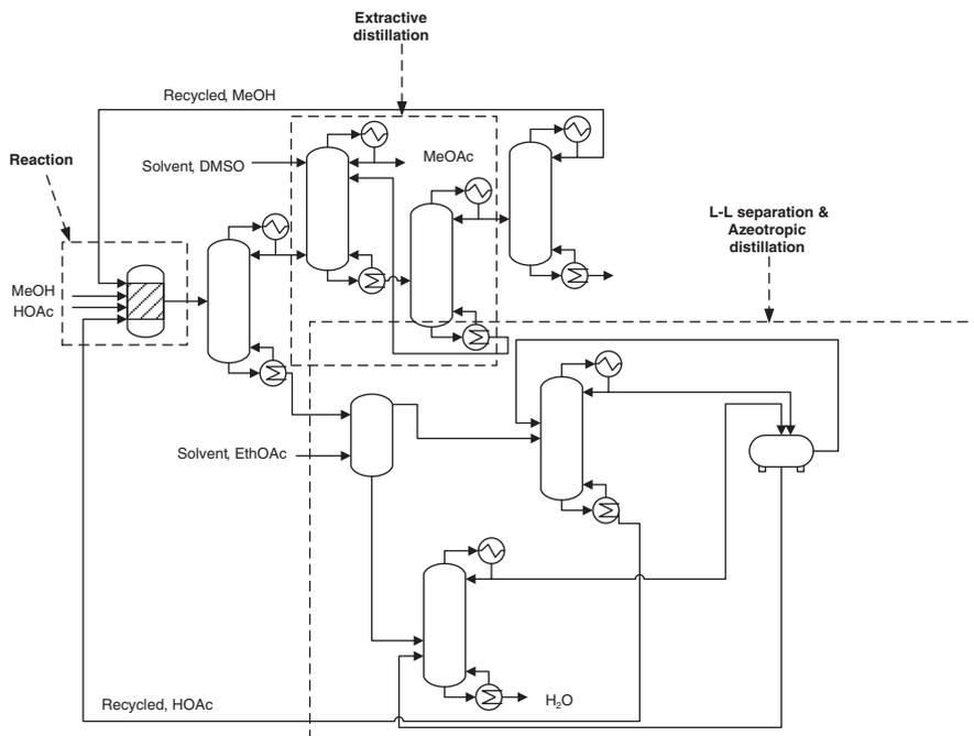
**Fig. 2.5** When to apply PI—process flowsheet for the production of methyl-acetate
