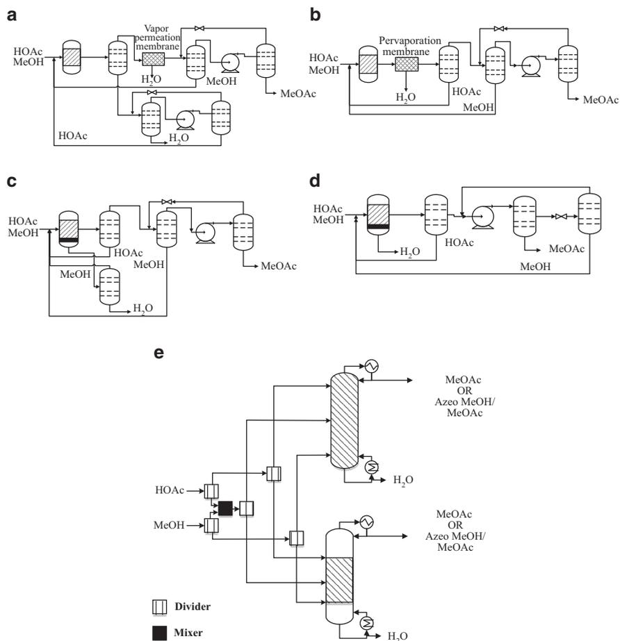
**Fig. 2.10** The generated flowsheet alternatives for the production of MeOAc [2]. (a) Flowsheet alternative 1, (b) Flowsheet alternative 2, (c) Flowsheet alternative 3, (d) Flowsheet alternative 4 (e) Flowsheet alternatives 6–9
