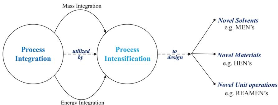
**Fig. 2.6** The utilization of process integration in process intensification. Examples of process intensification that employ mass and energy integration are shown. *MEN* mass exchanger network, *HEN* heat exchanger networks, *REAMEN* reactive mass exchanger network
