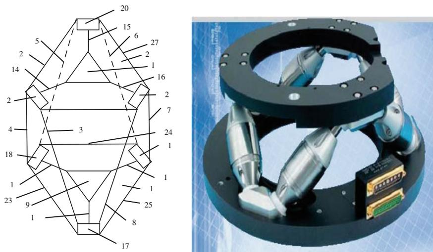
**Fig. 3** Driving hexapod design and its general appearance
