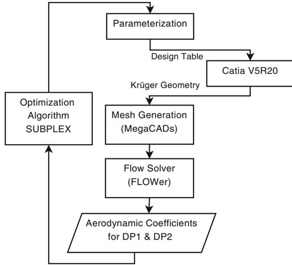
the optimization. The airfoil and Krüger shape are extracted in chord wise direction at the outboard position of the HLFC section. Afterwards the configuration is sweep scaled with the front-spar angle.
