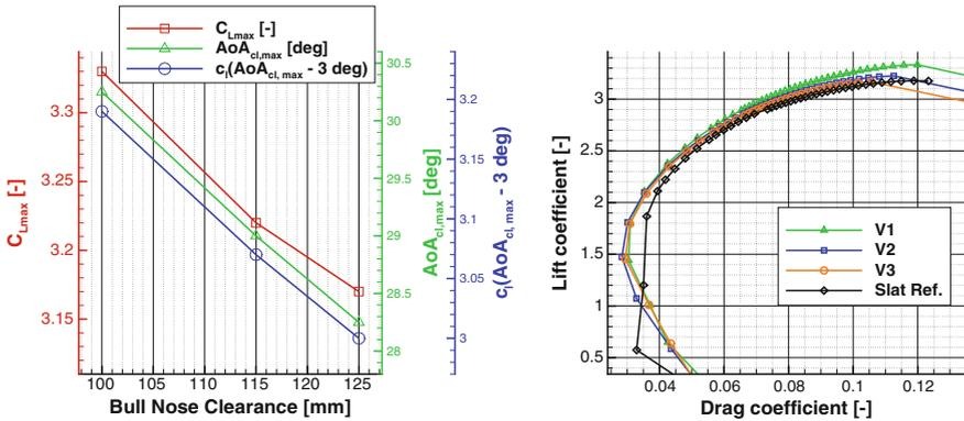
**Fig. 4** *left* Aerodynamic high-lift performance versus bull nose height clearance at DP1. *right*  $c_l$ - $c_d$  curve for optimized Krüger and reference slat configurations at DP1
