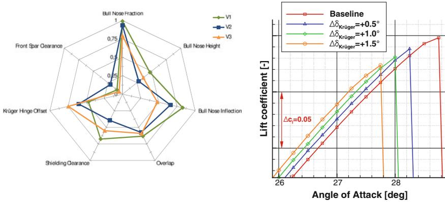
**Fig. 5** *left* Distribution of the values of the parameters for configuration V1–V3 with normalized design spaces. *right* Lift coefficient over angle of attack for deflection angle variation on intermediate Krüger device at DPI
