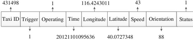
**Fig. 1.** Data format of a GPS data entry.
