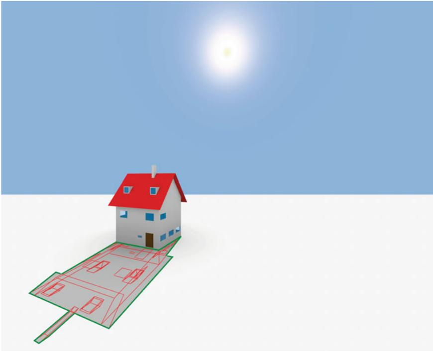
**Fig. 3** In our approach and our software implementation, the shadow on the ground is derived as a unionised set (*green*) of projected polygons (in *red*; 51 polygons in this LOD3 case) from the CityGML model, and accounting for the footprint
