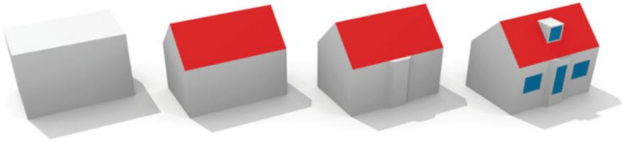
**Fig. 1** Our research in a nutshell: the estimation of the shadow differs between the different levels of detail, and the accuracy of the prediction seems to increase with each LOD. However, this should be investigated numerically and it is not straightforward as it may appear
