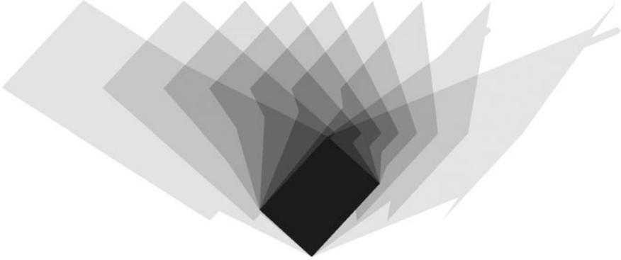
**Fig. 2** Orthogonal *top view* composite of 9 shadows during a day (also known as the butterfly shadow diagram; the *outline* of each shadow is drawn at hourly intervals) for an LOD3 model. It suggests the different degree of influence of LOD-related details on the shadow depending on the date, time, and location. The building footprint is shown in *black*
