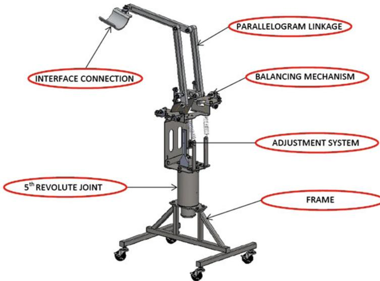
**Fig. 2** 3D CAD model and subcomponent labels
