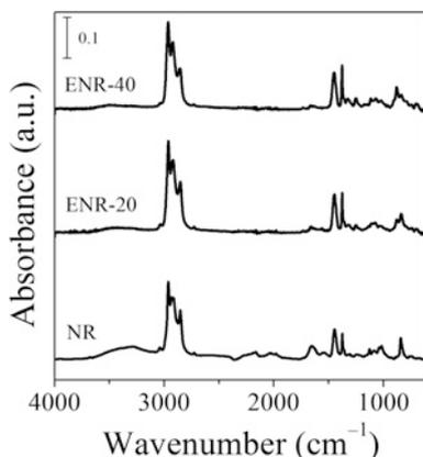
Fig. 2 FTIR spectra of NR and ENR
