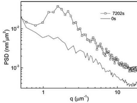
**Fig. 2.1** Power spectral density of an  $h_0 = 18$  nm and  $M_w = 2.3$  kg/mol spin-cast polystyrene film, freshly prepared (*plain solid line*) and after annealing for 7202 s (open squares) at 85 °C (Reproduced with permission from Ref. [13])
