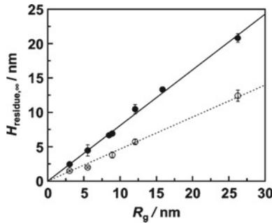
**Fig. 2.8**  $R_g$  dependence of the equilibrium residue thickness,  $h_{\text{residue},\infty}$  for residual films obtained from PS/H-Si (solid circles) and PS/SiO<sub>x</sub>-Si (open circles). In this plot, the value of  $R_g$  is deduced from the weight average molecular weight of the polymer (Reproduced with permission from Ref. [33])
