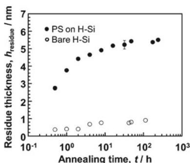
**Fig. 2.7** Annealing time dependence of the thickness of the residual film,  $h_{\text{residue}}$  obtained from PS/H-Si (solid symbols) and bare H-Si (open symbols). The annealing was carried out at 150 °C in air. The PS has  $M_w = 44.1$  kg/mol and initial thickness,  $h_0 = 200$  nm (Reproduced with permission from Ref. [33])
