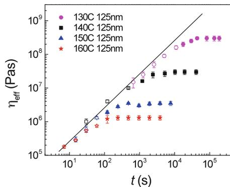
**Fig. 2.5** Effective viscosity  $\eta_{\text{eff}}$  versus time obtained from PS-SiO<sub>x</sub> films with  $h_0 = 125$  nm films annealed at various temperatures between 130 and 160 °C. The *solid line* is a plot of  $\eta_{\text{eff}} = 2 \times (10.5 \text{ kPa}) \times t$  (Data reproduced with permission from Ref. [40])
