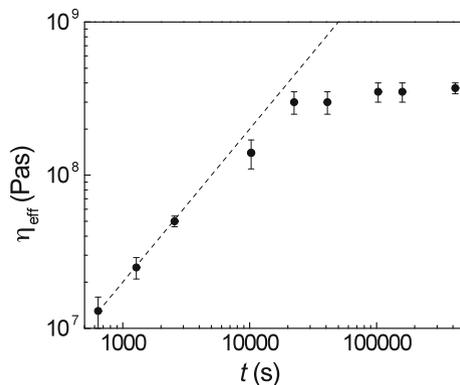
**Fig. 2.4** Values of  $\eta_{\text{eff}}$  obtained by fitting the PSDs in Fig. 2.3 one-by-one to (2.1a, 2.1b), plotted versus the annealing time,  $t$ . The *dashed line* is a plot of  $\eta_{\text{eff}} = 2\mu_0t$  (Reproduced with permission from Ref. [41])
