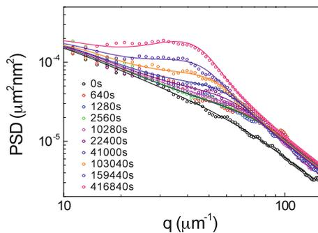
**Fig. 2.3** Power spectral density of a  $h_0 = 3$  nm,  $M_w = 115$  kg/mol PS film upon annealing at  $115^\circ$  C for various times as shown in the legend (*open circles*). The *solid lines* are model lines obtained by fitting the data to (2.4a), which gives  $\eta_{\text{eff},0} \equiv h_0^3/(3M_{\text{tot}}) = 4.2 \times 10^8$  Pas and  $\mu_0 = 10$  kPa (Reproduced with permission from Ref. [41])
