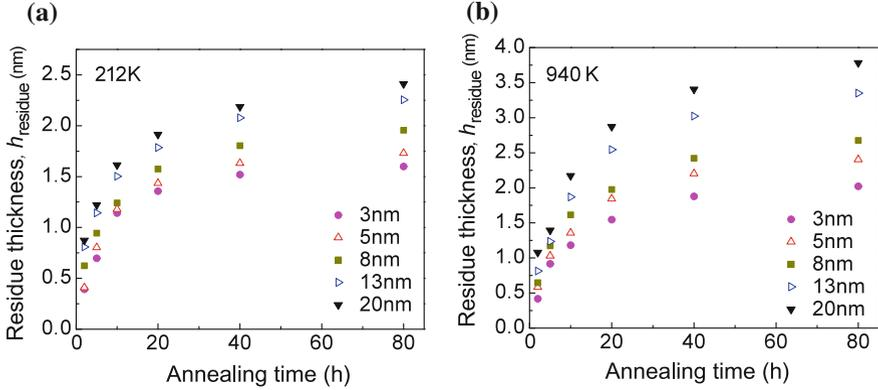
**Fig. 2.10** Temporal evolution of  $h_{\text{residue}}$ , the thickness of the adsorbed layer produced from PS spun-cast on silica with various initial thicknesses. **a** Data taken from films with  $M_w = 212$  kg/mol and **b** 940 kg/mol. The annealing temperature was 120 °C. The initial thicknesses are as shown in the legend
