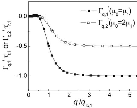
**Fig. 2.6** An illustration of the effect of doubling  $\mu_0$  on  $\Gamma_{q'}$ . The vertical axis is normalized by  $1/\tau_{r,1} \equiv \lim_{q \rightarrow \infty} \Gamma_{q,1}'$ , the original limiting value before  $\mu_0$  is doubled. The horizontal axis is normalized by  $q_{lc,1}$ , the original lower cut-off wavevector of the elastic-state or “rubbery” PSD
