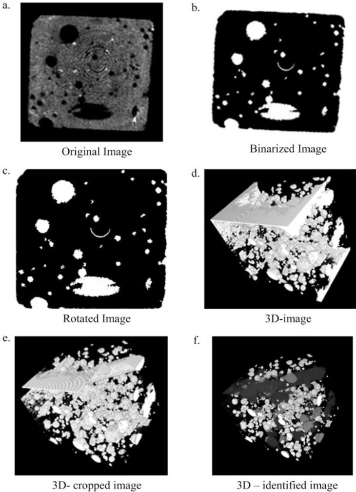
**Fig. 2** Steps of the lightweight mortar mixture analysis methodology. In the figure, the sample contains mortar, fibers, and EVA
