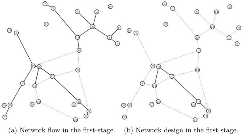
**Fig. 3** First-stage decisions: network flow ( $x$ ) and network design ( $\delta$ ).
