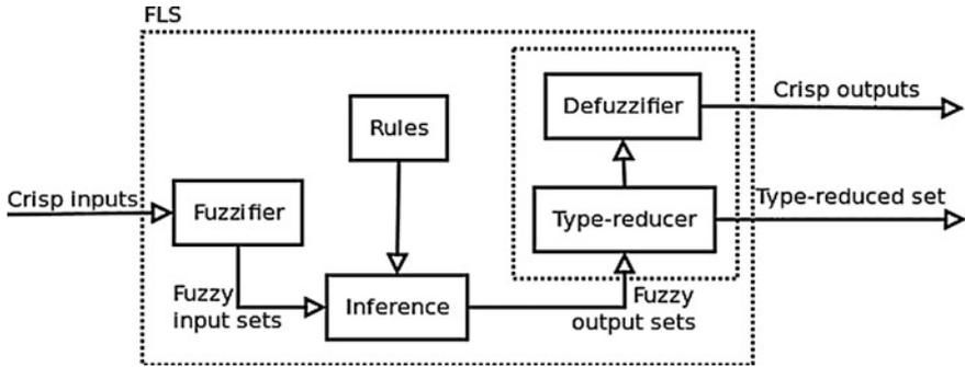
**Fig. 1** Block diagram describing an IT2 FLS. With a crisp input, two outputs are possible, a confidence interval in which any possible point within such interval is a correct answer, or a crisp value, in the case a single real number is required as output
