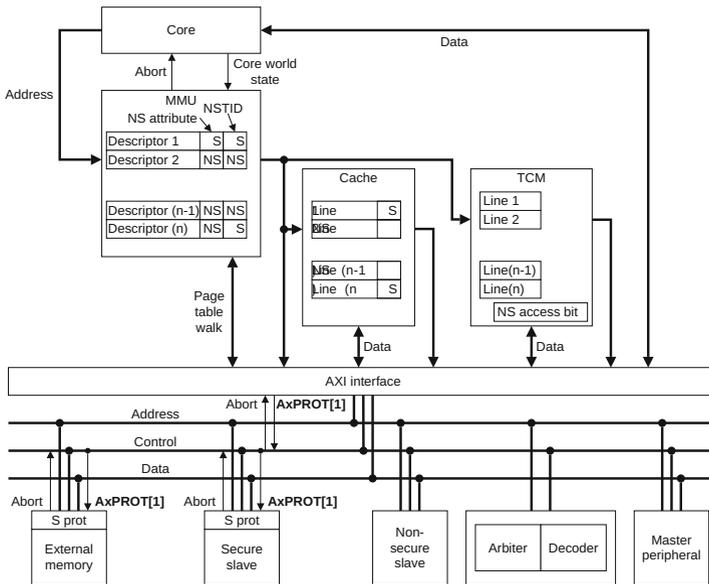
**Fig. 4.** ARM architecture with TrustZone extensions: propagation of the normal (NS=1) and secure (NS=0) signal (AxPROT) system-wide via bus transactions. Source: <http://infocenter.arm.com/help/index.jsp?topic=/com.arm.doc.ddi0333h/Chdfjdgi.html>
