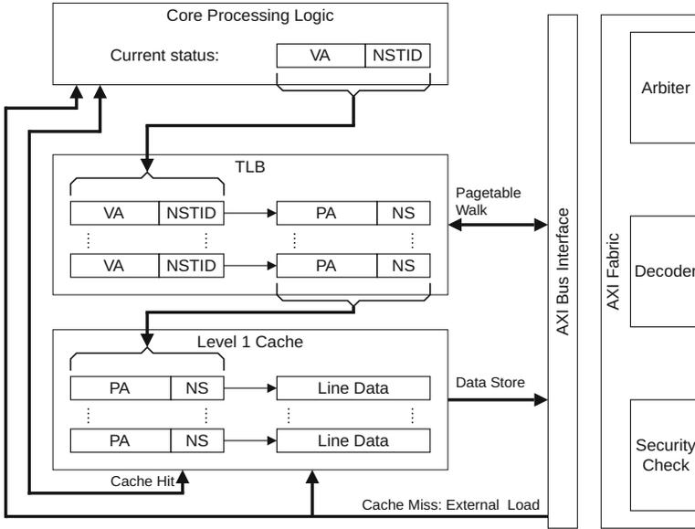
**Fig. 5.** ARM architecture with TrustZone extensions: cache logic with respect to the normal (NS=1) and secure (NS=0) worlds. Source: <http://infocenter.arm.com/help/index.jsp?topic=/com.arm.doc.prd29-genc-009492c/ch03s03s02.html>
