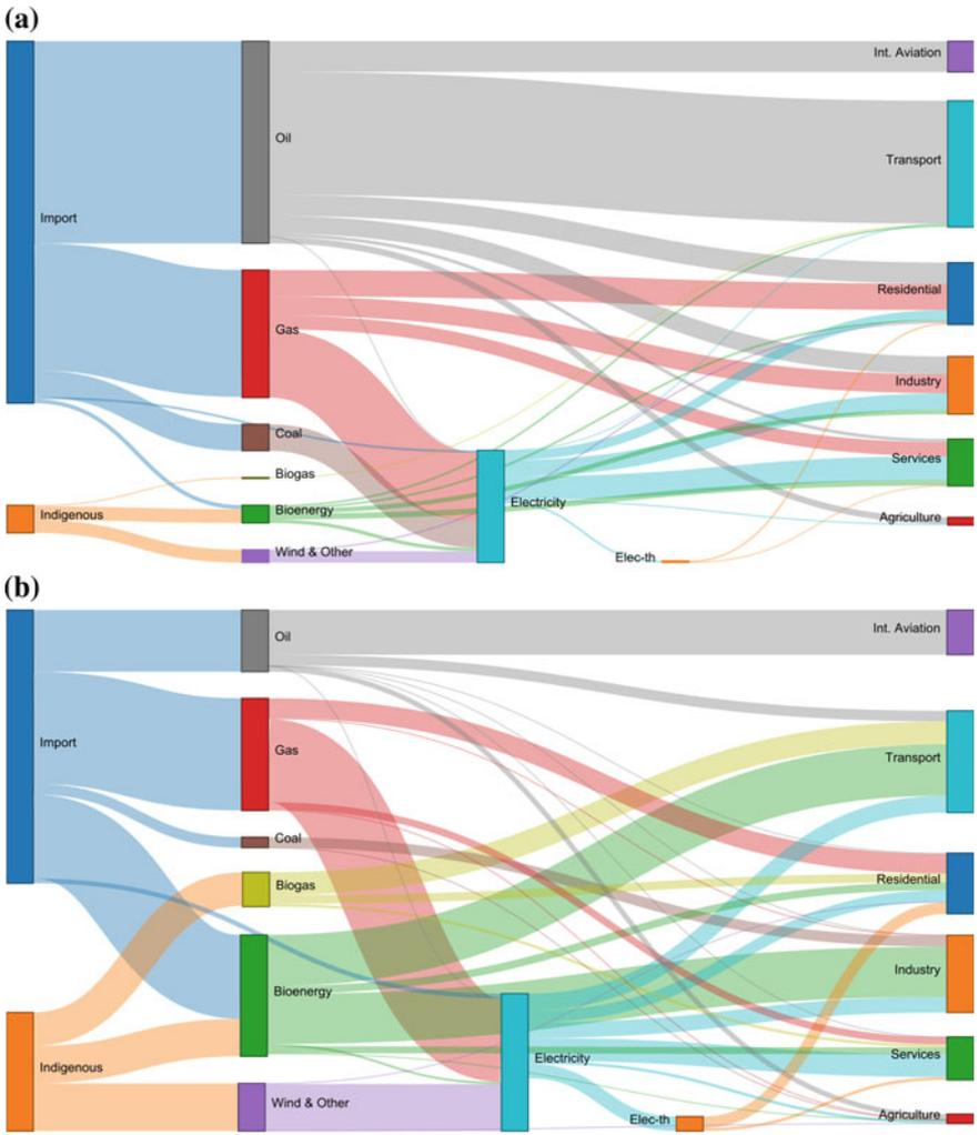
**Fig. 2** 2050 Sankey Diagrams for Ireland’s energy system under BaU, CO<sub>2</sub>-80 and CO<sub>2</sub>-95 scenarios. **a** BaU scenario. **b** CO<sub>2</sub>-80 scenario. **c** CO<sub>2</sub>-95 scenario
