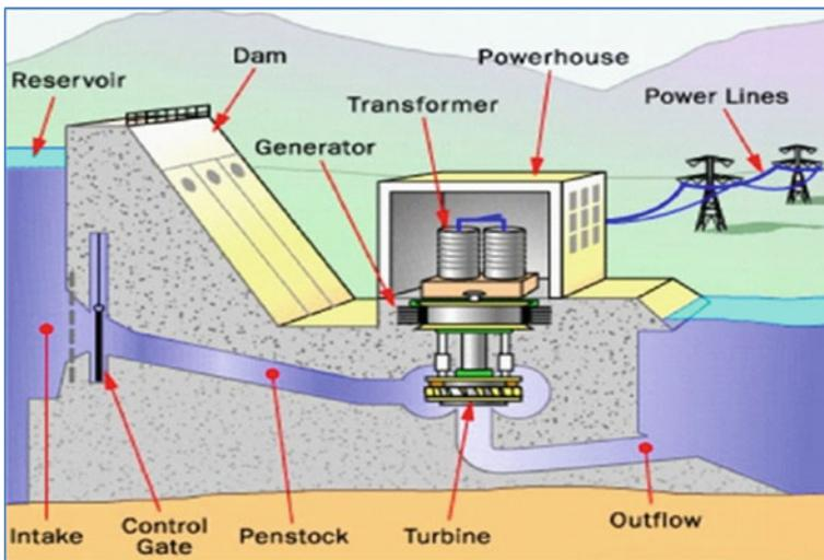
Fig. 2.4 A view from *inside* part of reservoir hydropower plant (from HowStuffWorks 2001)
