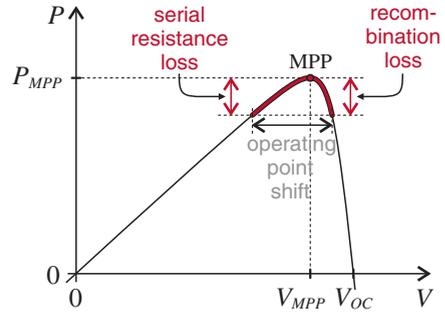
mismatch is lost either as a Joule power dissipation on serial resistances when the device segment's voltage is reduced (marked as serial resistance loss in Fig. 2.3) or as a Joule power dissipation by non-radiative recombinations and a radiation emission by radiative recombinations when the device segment's voltage is increased (marked as recombination loss in Fig. 2.3).
