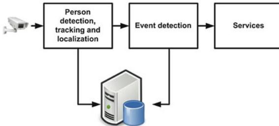
**Fig. 1** Overall of vision-based person surveillance system
