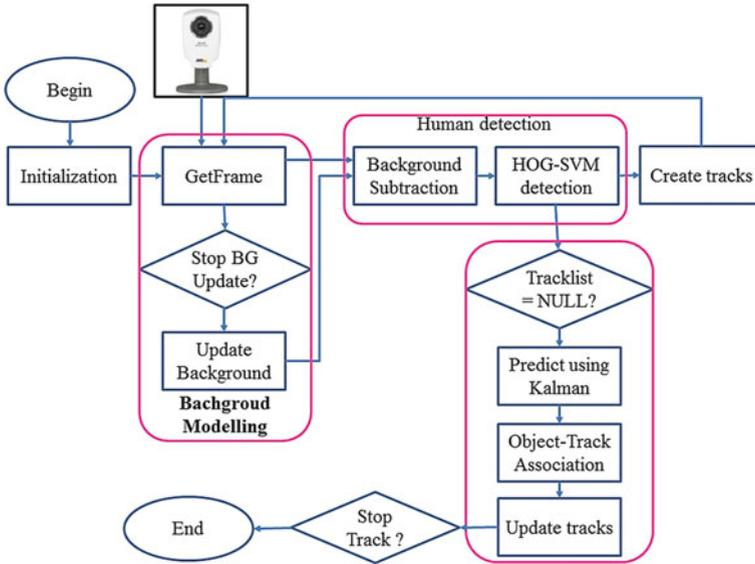
Fig. 2 Diagram of object detection and tracking
