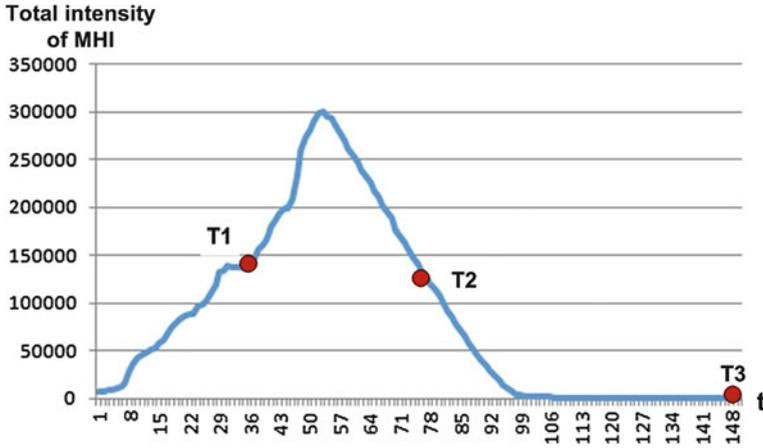
**Fig. 8** Illustration of total value of MHI computed for a sequence of human activity: walking (from 0 to T1), falling (from T1 to T2) and being motionless on the floor (from T2 to T3)
