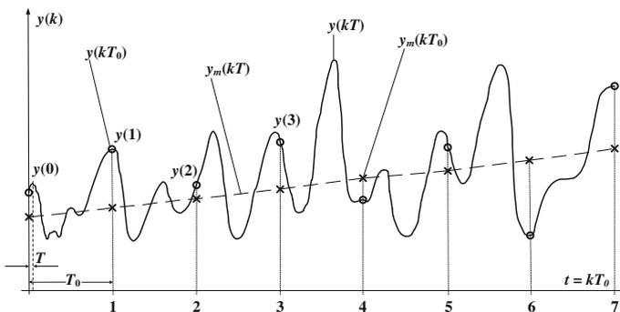
**Fig. 4** The vibration signal (1 min sampling time)
