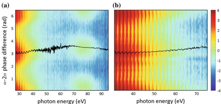
**Fig. 2** Scan of harmonic spectra acquired in xenon (a) and krypton (b) as a function of photon energy and two-color phase difference (log scale). The *black line* corresponds to the phase of the spectral oscillation retrieved by Fourier transforming the sequence of harmonic spectra for each photon energy and by selecting the component at the oscillation frequency
