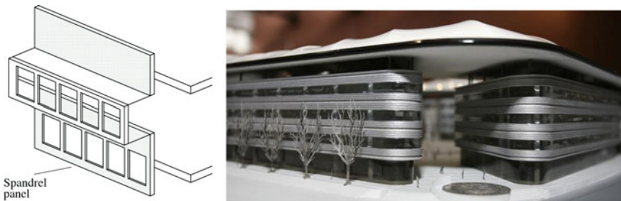
Fig. 2.10 Spandrel ribbon curtain wall systems
