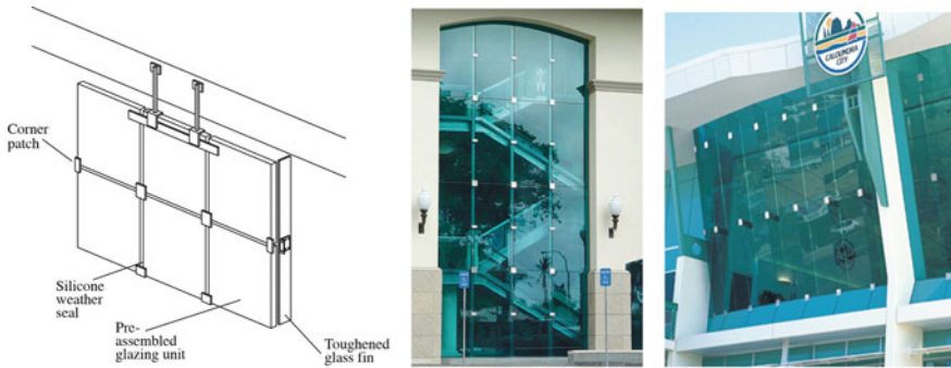
Fig. 2.13 Patch structural glazing
