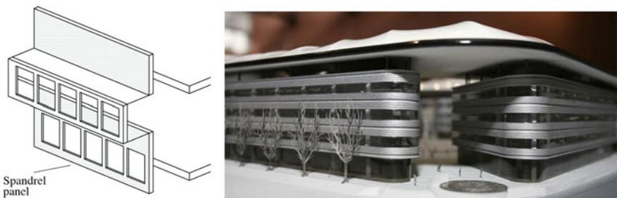
**Fig. 2.10** Spandrel ribbon curtain wall systems
