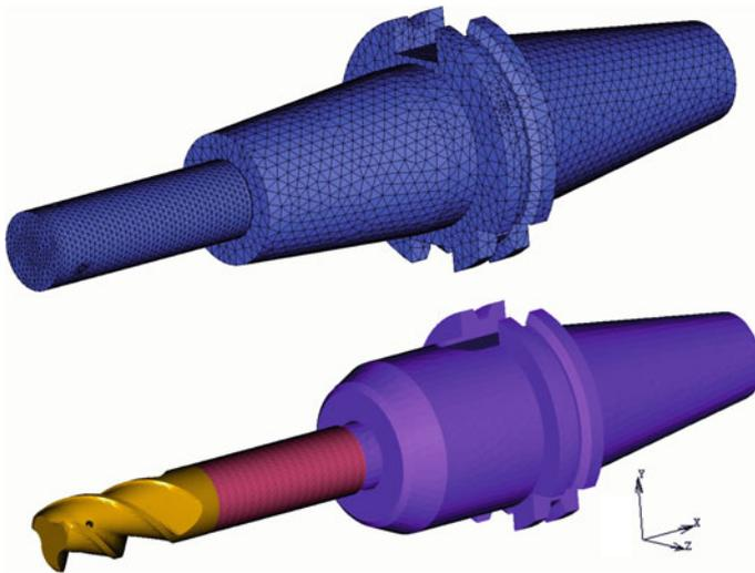
**Fig. 2.3** Exemplary FE models—tool and chuck models (*top* dummy tool in shrink-fit chuck, *bottom* end mill and chuck with clamping surface, separated representation)
