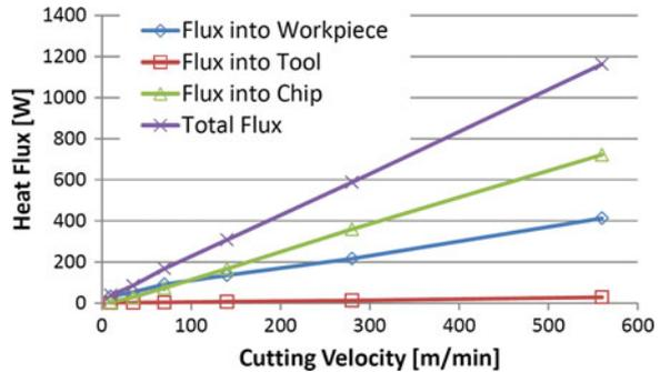
**Fig. 2.10** Heat flow distribution in per cent, calculated for different cutting speed values
