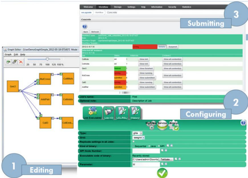
Fig. 2.2 The three generic workflow development phases in WS-PGRADE
