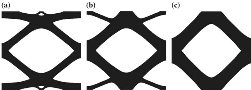
**Fig. 10** Example 6. Shear modulus and horizontal conductivity maximization. **a**  $\beta = 0.25$ , **b**  $\beta = 0.50$ , **c**  $\beta = 0.75$
