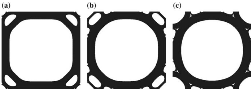
**Fig. 6** Example 2. Bulk modulus and orthogonal conductivity maximization. **a**  $\beta = 0.25$ , **b**  $\beta = 0.50$ , **c**  $\beta = 0.75$
