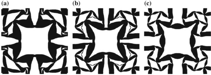
**Fig. 9** Example 5. Poisson ratio minimization and orthogonal conductivity maximization. **a**  $\beta = 0.25$ , **b**  $\beta = 0.50$ , **c**  $\beta = 0.75$
