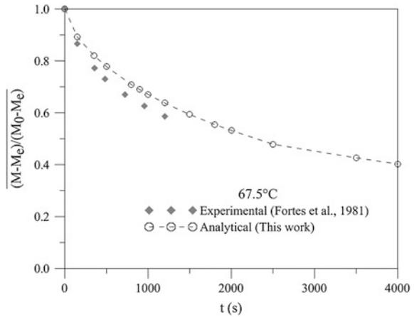
**Fig. 8** Dimensionless temperature at the center of the wheat grain as a function of time
