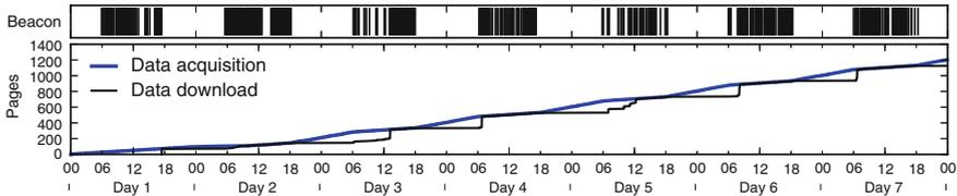
**Fig. 3** Timeline of received radio announcement packets at the base station from a single bat (*top*) and the number of generated versus downloaded flash pages (*bottom*)
